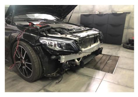
Suggested place for 12V power supply and fuse, Gnd to Car Body
