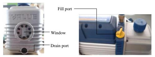
Note: the new vacuum pump oil cannot be filled too much into the vacuum pump otherwise it will spray out when working.
